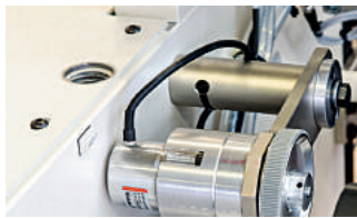
Load cell tension control.
